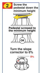
Place a pedestal on various places on the ground to determine the value of the slope
